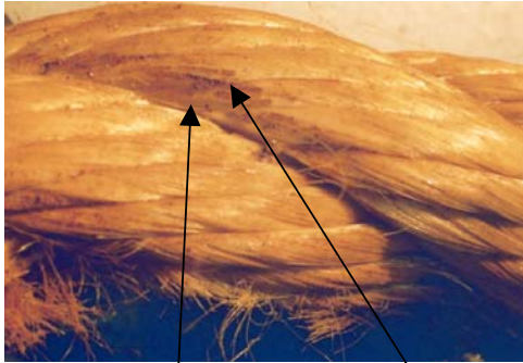
Figure 8. A close up photograph of figure 7 revealed abrasion failed filament ends. It can also be seen that there was negligible inter-strand abrasion inter-strand at this same region. There was some rust deposit on the strand and it was suggested this may have accelerated the abrasion. However, the absence of inter-strand abrasion proves this theory not to be possible.
