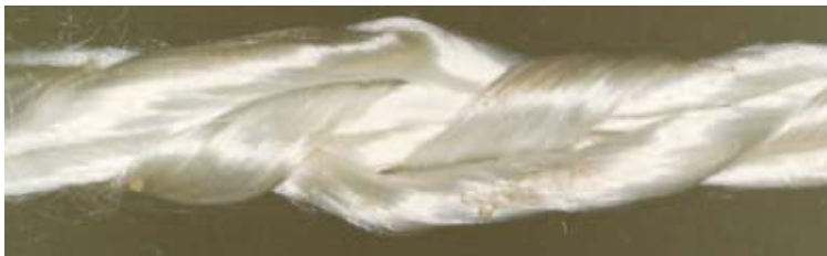
Figure 12. An examination of the sub-rope splice revealed no inter-strand abrasion at all in the clear rope
