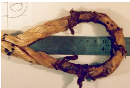
Figure 6. Intact eye with single layer of Dyneema cloth wrapped in a spiral direction around the eye. The Dyneema cloth had not worn through on the stainless steel spools.
