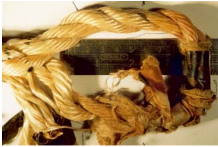
Figure 5. One strand failed at the tangent contact of the eye on the spool
