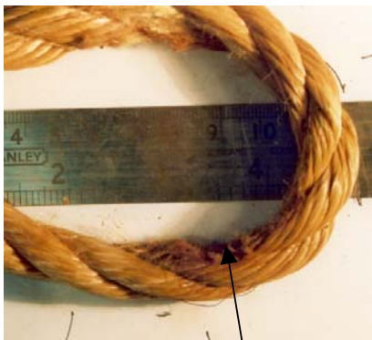
Figure 7. When the cloth was removed as shown in figure 6, the eye had severe abrasion damage around the contact on the spool with the maximum damage on the rope in the sliding zone at the tangent contact on the spool. The outside layer of yarn in the strand had virtually completely worn through.
